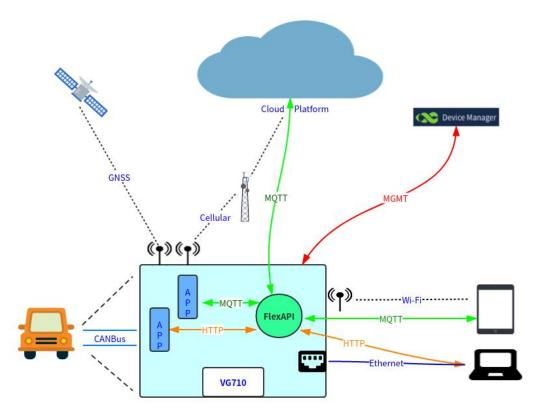
In the above figure, our VG710 at the central part physically connects to the vehicle, GNSS satellites, cellular base station, cloud platforms, Wi-Fi equipped tablet and Ethernet equipped industrial PC. Besides, service data stream flow from FlexAPI to cloud platform, local Python/Docker APPs and LAN device software.
